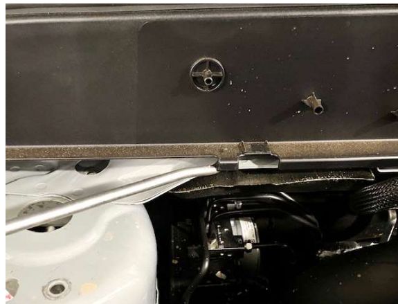
Step 9. Using a 10mm socket, remove plastic panel covering strut bolts.
