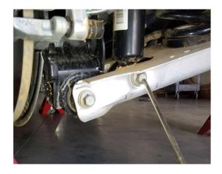
Step 10. Remove bolt holding lower control arm to wheel hub.
