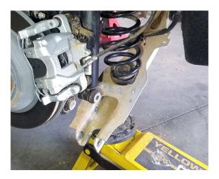
Step 12. Remove spring and upper rubber isolator.
