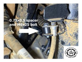
Step 20. Install lower bolt connecting strut to knuckle.
