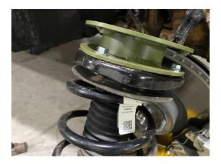
Step 18. Reinstall strut with spacer attached, using original hardware through the shock tower and into the spacer.
