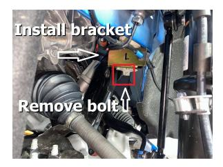
Step 16. Reroute ABS wire as shown brake line bracket and plug back into wheel sensor. (see photo)
