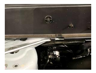
Step 7a (HYBRID MODELS ONLY) unclip wiring harness from cowl cover.
